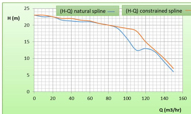
**Figure 6:** Numerical results for (H-Q) curve to parallel connection of pumps with different characteristics.
