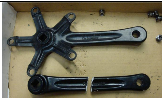
Figure 1: Typical bike crank arm failure due to fatigue
