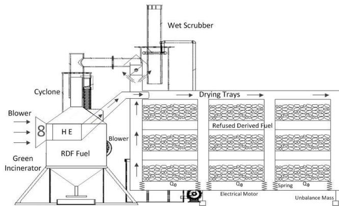
**Figure 5:** RDF dryer machines by using Vibration Components, Heat Exchanger, Micro Hydro Power Plant and Green incinerator.
