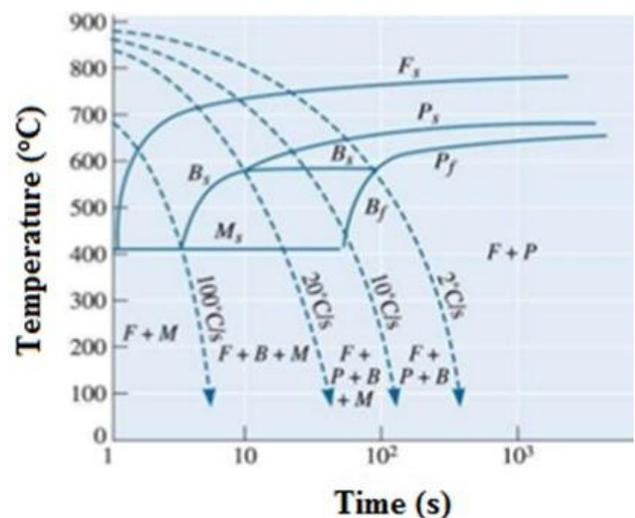
Figure 1: CCT diagram of 0.2% C [9]
