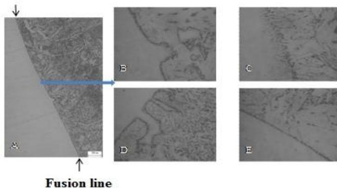
**Figure 6:** (A) Microstructures at the fusion line, (B) island, (C, E) beach, (D) peninsula
