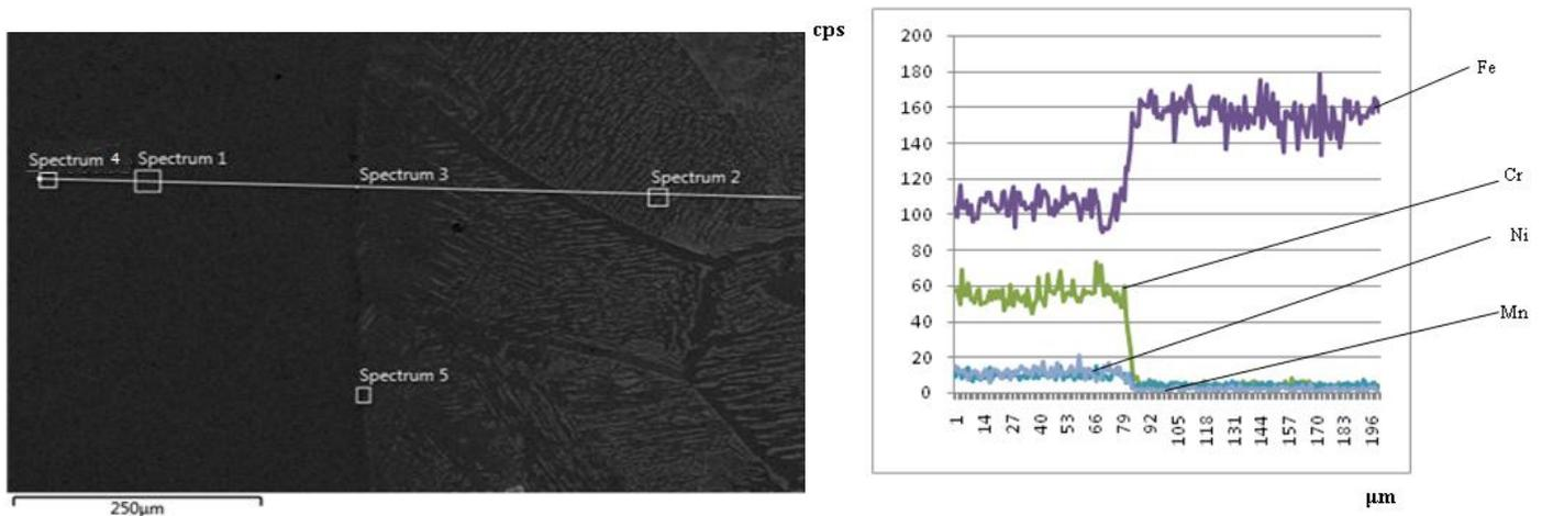
Figure 4: Elements distribution profiles in the transition zone
