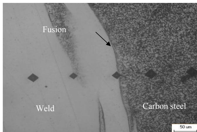
**Figure 8:** Microstructures of hardness test
