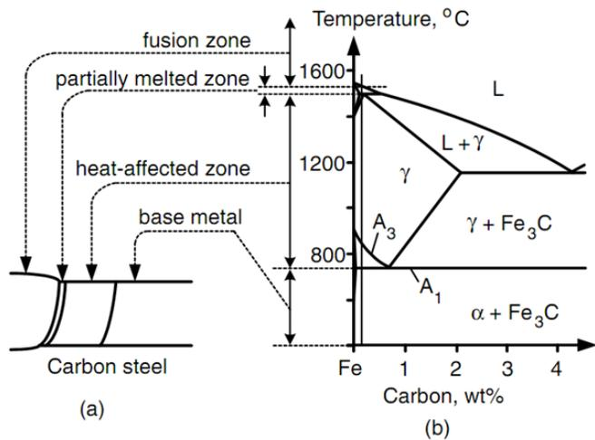
**Figure 2:** The microstructure of the weld
