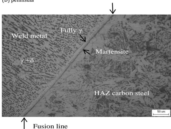
**Figure 7:** Microstructures in the transition zone
