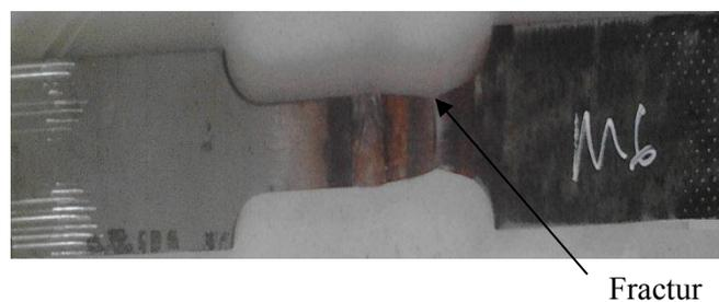
**Figure 9:** Tensile test sample
