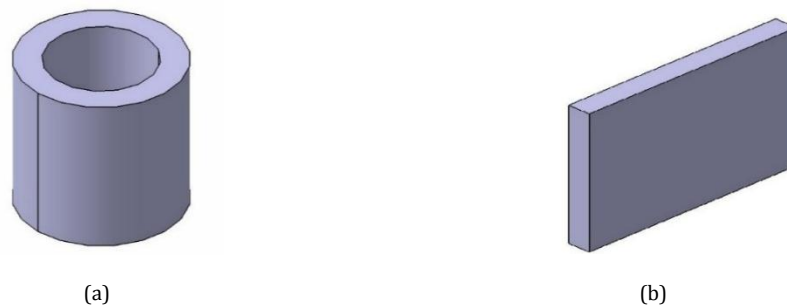
Figure 5: CATIA drawing of the two specimens (a) Custom cylinder for first experiment (b) Rectangular design for the second experiment
