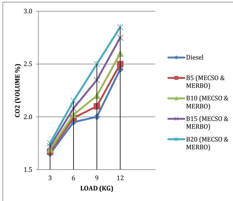
Figure 3: Variation of CO<sub>2</sub> with Load for Different Blends at CR18
