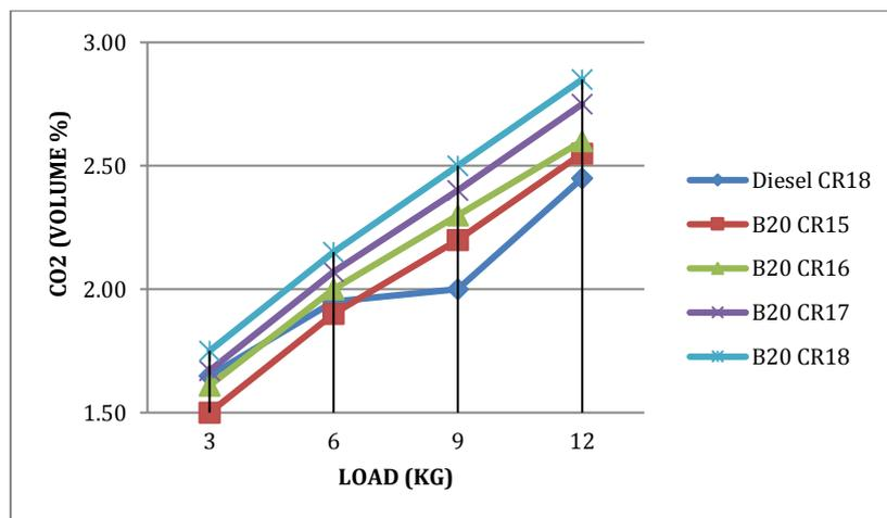
Figure 4: Variation of CO<sub>2</sub> with Load for Different CRs with Diesel and B20 Blends
