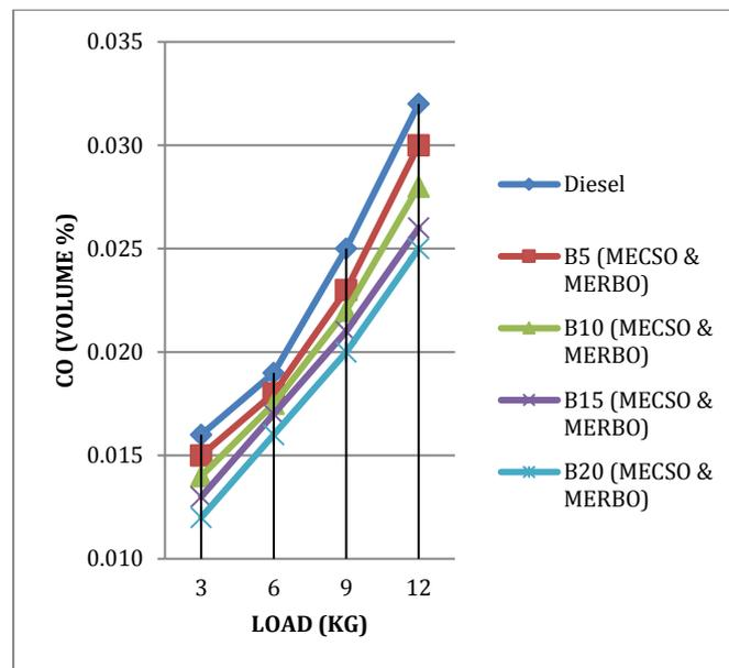
Figure 1: Variation of CO with Load for Different Blends at CR18
