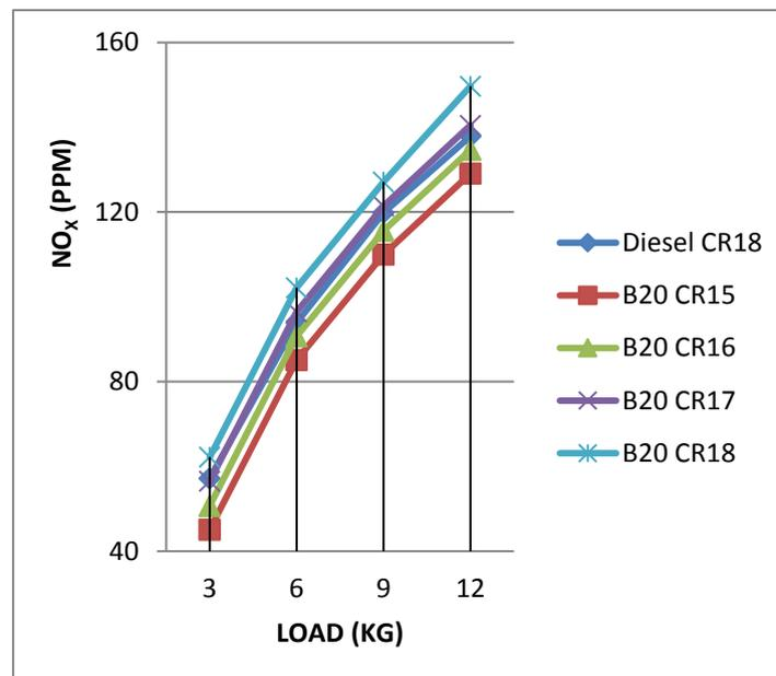
Figure 7: Variation of NO<sub>x</sub> with Load for Different CRs with Diesel and B20 Blends
