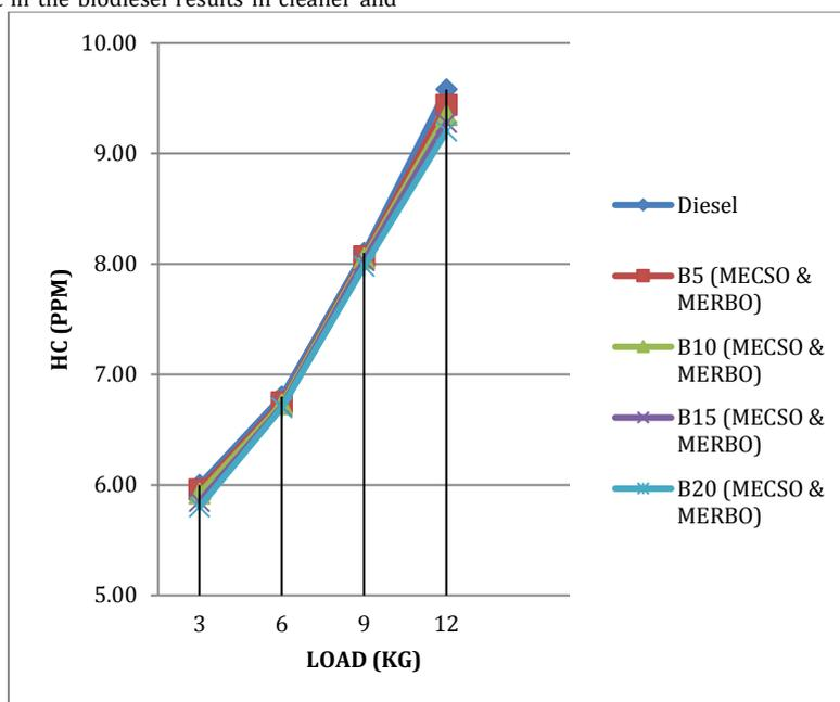
Figure 5: Variation of HC with Load for Different Blends at CR18
