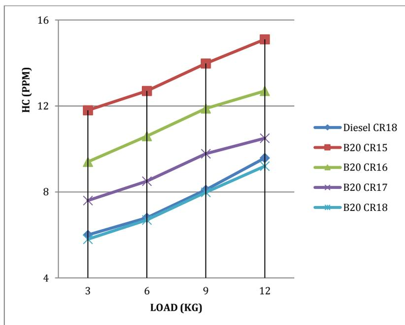
Figure 6: Variation of HC with Load for Different CRs with Diesel and B20 Blends
