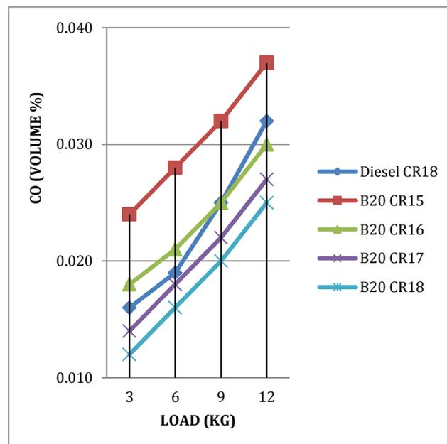
Figure 2: Variation of CO with Load for Different CRs with Diesel and B20 Blends
