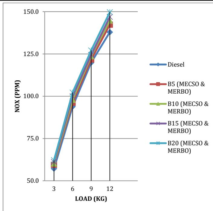
Figure 6: Variation of NO<sub>x</sub> with Load for Different Blends at CR18
