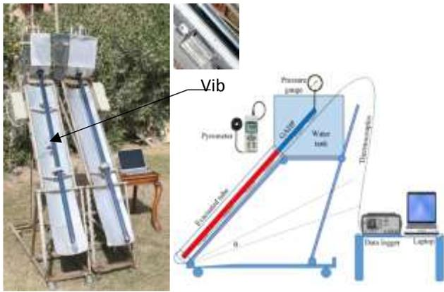
**Figure 1:** Experimental rig setup and schematic diagram for HP-ETSC with and without vibrator.
