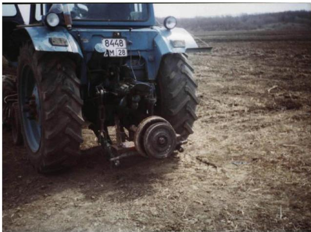
**Figure 2:** Tractor with an optional flywheel
