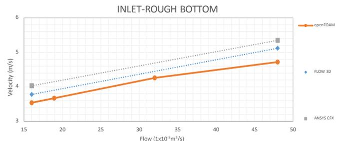
**Figure 5:** Results of all simulations for rough bottom in the outlet of a chute
