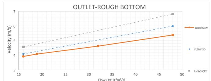
**Figure 4:** Results of all simulations for a rough bottom in the inlet of a chute
