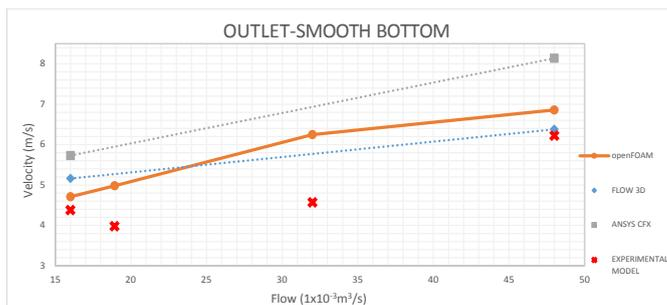
**Figure 3:** Results of all simulations for a smooth bottom in the outlet of a chute
