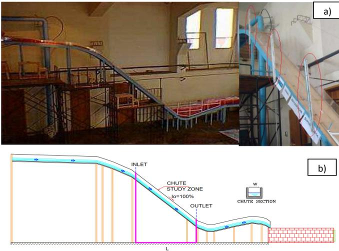
**Figure 1:** a) Chute Hydraulic Model 1:25 "El Batán" Creek, b) Chute Hydraulic Model 1:25 "El Batán" Creek
