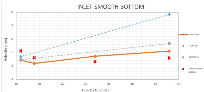
**Figure 2:** Results of all simulations for a smooth bottom in the inlet of a chute
