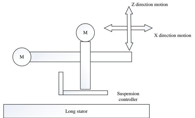
Figure 4: Special signal loading mechanism for suspension guide sensor
