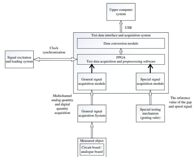
Figure 5: Debug data interface and acquisition system
