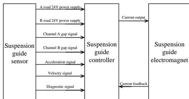
Figure 1 : signal transmission diagram of a suspension guide sensor
