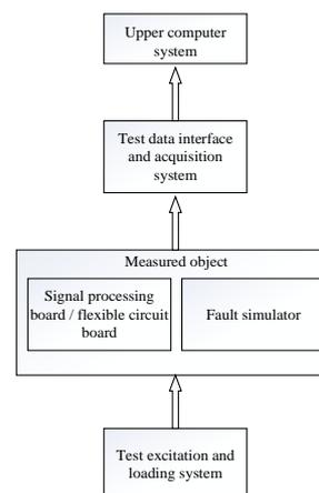
Figure 2 : Structure of fault location device for suspension guiding sensor
