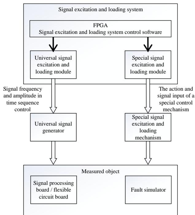
Figure 3: Test excitation and loading system
