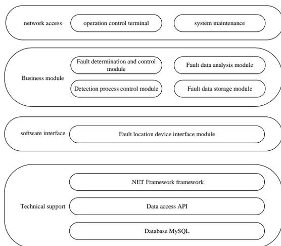
**Figure 6:** Software system diagram of fault location device for suspension guiding sensor
