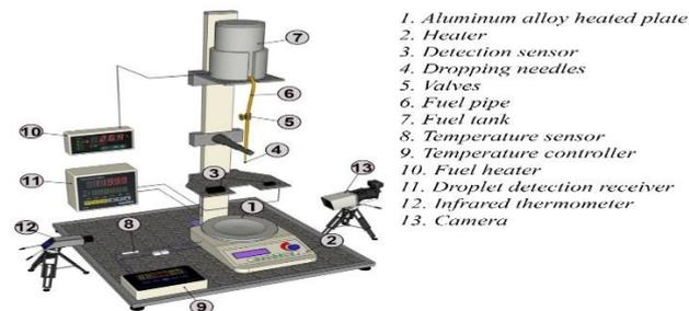
Figure 1: Test diagram about deposits formation on the heated wall surface
