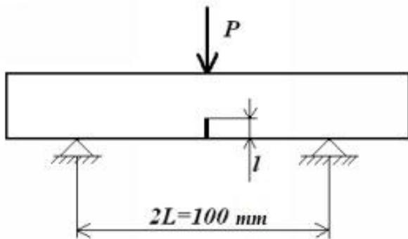
**Figure 2:** Scheme of loading of a specimen with a notch for a three-point and a point
