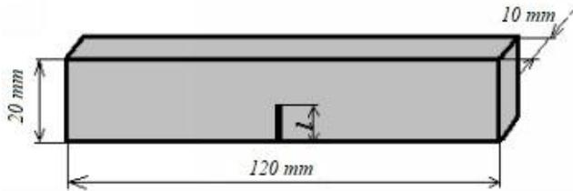
**Figure 1:** Sample with a notch for 3-point bending tests to determine the crack resistance characteristics of the CAS
