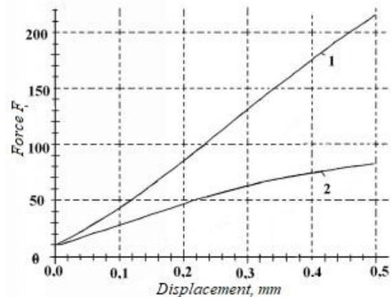
**Figure 3:** The experimental dependence of the concentrated force  $P$  on the displacement  $\delta$  of samples with different notch sizes:  $l$  - 5 mm, 2-12 mm
