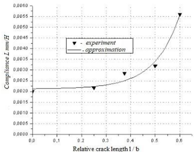
**Figure 4:** Dependence of compliance  $l$  of the relative crack length  $l/b$
