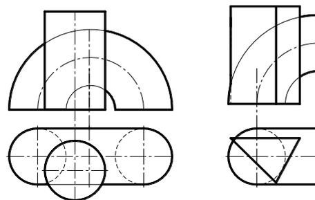
**Figure 4:** Intersection lines of the surfaces
