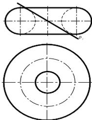
**Figure 2:** A line of intersection of the open torus with the front-projecting plane P
