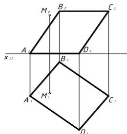
**Figure 1:** The point and its reflection are symmetric with respect to the plane of the mirror
