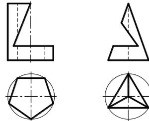
**Figure 3:** A profile projection of the surfaces with the given cut-outs
