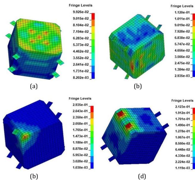
**Figure 5:** Effective (Von Mises) stress distribution on the 2 m drop height: (a) Flat Position; (b) 45-degree X-axis rotation; (c) Corner side rotation; (d) Connector side drop
