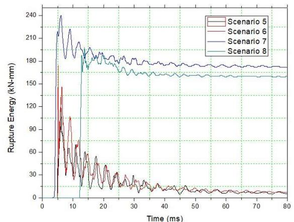
**Figure 8:** The absorbed rupture energy of modular pontoon unit on 4m height drop
