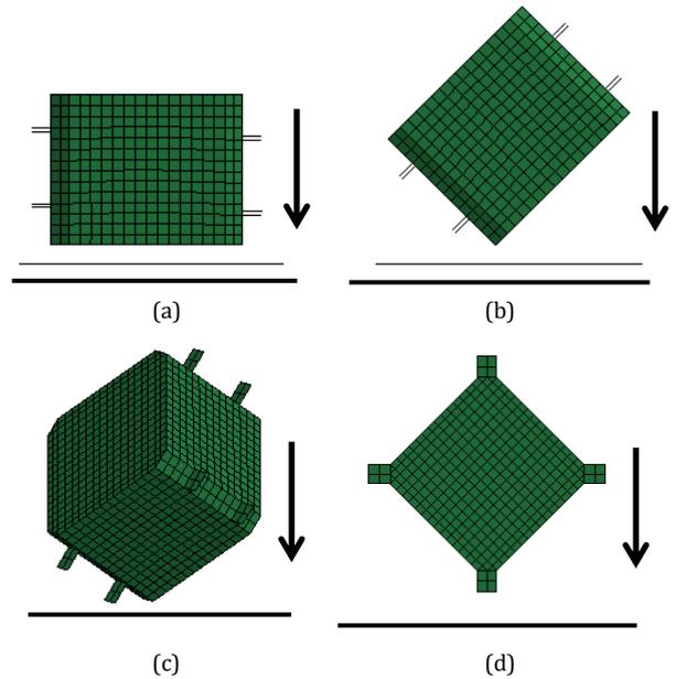
**Figure 4:** Drop test orientation: (a) Flat Position; (b) 45 degree X-axis rotation; (c) Corner side; (d) Connector side drop
