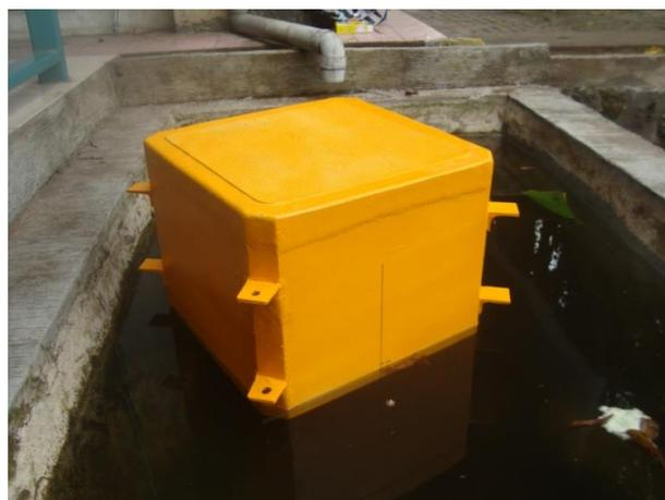
**Figure 3:** GFRP Modular Pontoon Unit
