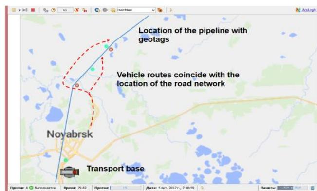
**Figure 4:** Simulation of the movement of equipment to the place of oil pipeline repair on the existing road network
