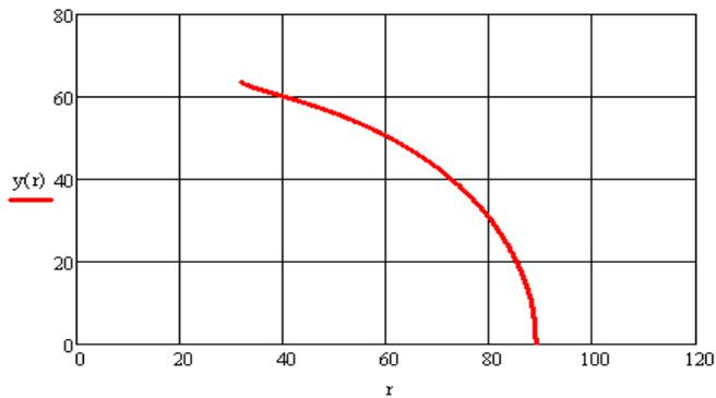
**Figure 3:** The profile of the bottom of the water filter tank is made of the composite after calculation
