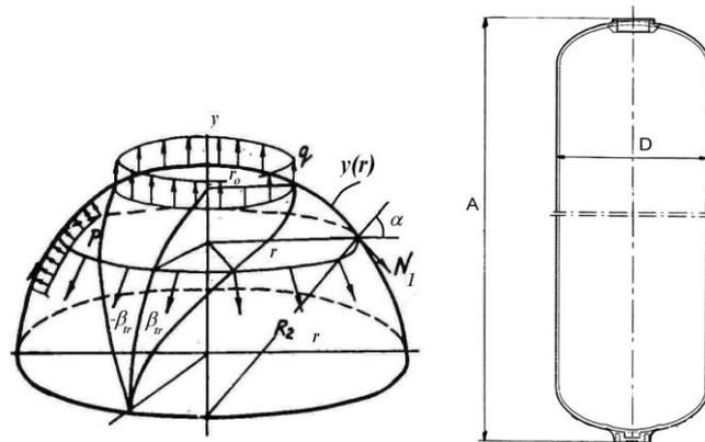
Figure 1: Model of calculating the cylinder
