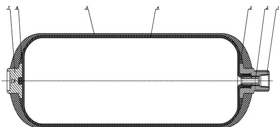
**Figure 2:** Structure of the composite water filter tank with sealed plastic cover: 1- connecting valves (neck cylinders), 2-taper, 3- 6-section stress relief, 4-sealed housings from HDPE, 5-pressure bearing from composite, 7-bottomed
