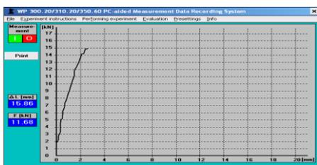
**Figure 10:** Strength curve after tempering 2h
