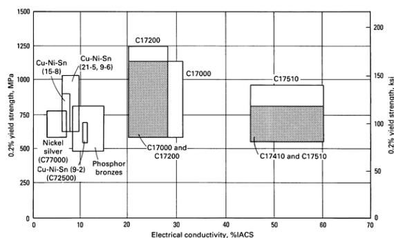
Figure 1: Strength and electrical conductivity for copper alloys
