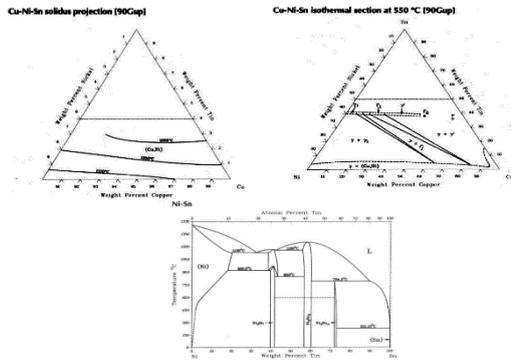
**Figure 2:** The cross-section diagram of Copper-nickel-tin alloy
