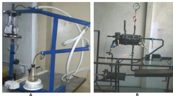
**Figure 4:** Laboratory installations for obtaining oil solvents: A – base; B – aromatized
