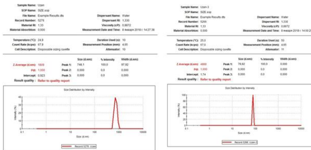
Figure 12: The intensity of the size distribution of solid suspended particles in the water injected into the reservoir before and after cleaning
