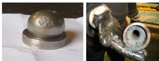
Figure 4: Wear class pair due to admission to the pump of mechanical impurities
