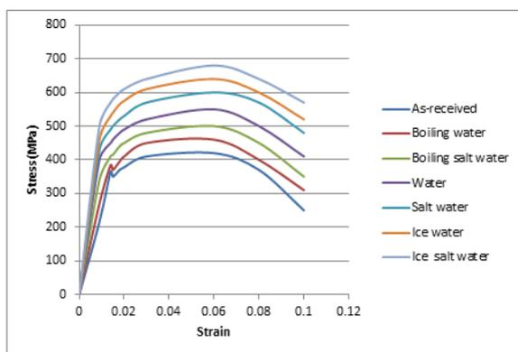
Figure 3: Relationships between stress-strain curves for all the specimens treated in different quenching media
