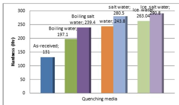
Figure 4: Relationships between hardness and quenching media
