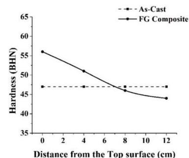
Figure 3: Hardness of Al-Si FG composite along the length of the cast
