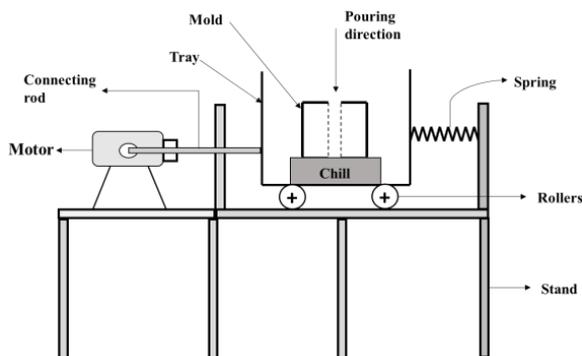
Figure 1: Lateral vibration experimental set up
