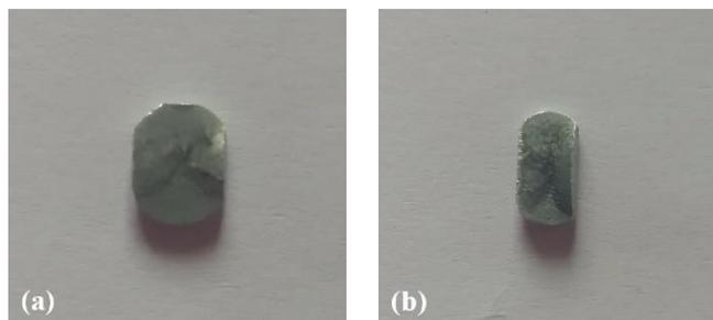
**Figure 4:** Diametrical compression (a) Top portion (b) Bottom portion
