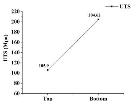
**Figure 5:** Ultimate tensile strength at top and bottom portion of the cast
