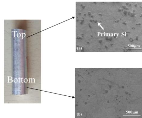
Figure 2: SEM micrographs of FG Composite a)top portion b)bottom region
