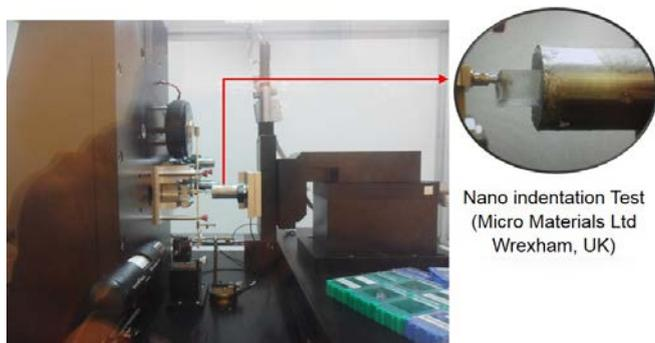
Figure 2: Experimental setup for nanoindentation test
