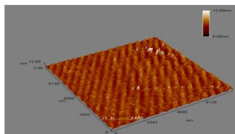
Figure 3: AFM micrograph of the prepared SSNPs
