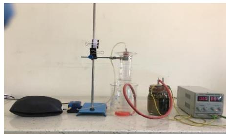
Figure 2: Hydrogen Generator
