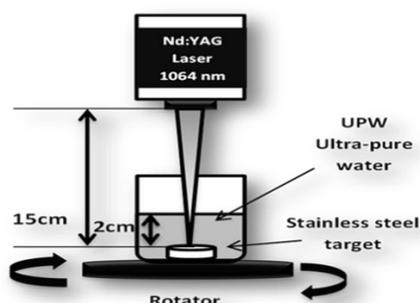
Figure 1: Scheme of the modified PLAL system
