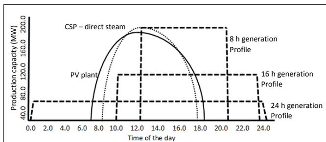
**Figure 2:** Production scenario of integrated solar plants with energy storage
