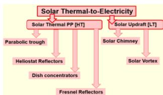
**Figure 1:** Classification of solar thermal power technologies.
