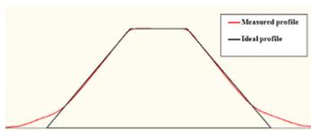
**Figure 7:** Deviation between measured and ideal model(D=10mm,  $\alpha=50^\circ$ ,  $\Delta z=0.6\text{mm}$ )
