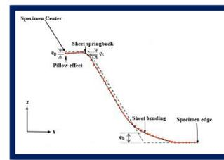
Figure 2: Type of geometrical errors. [3]
