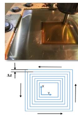
Figure 3 : Incremental sheet forming with tool path
