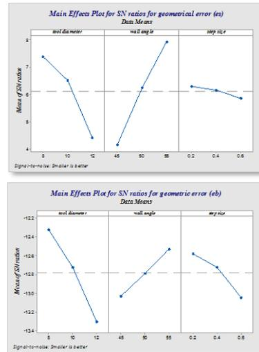
Figure 5: Mean effect plot for S/N for geometrical error.
