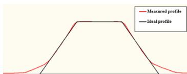
**Figure 8:** Deviation between measured and ideal model(D=12mm,  $\alpha=55^\circ$ ,  $\Delta z=0.4\text{mm}$ )
