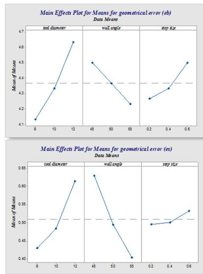
Figure 4: Mean effect plot for mean for geometrical error.
