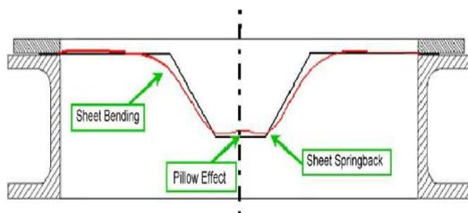
Figure 1: Different geometrical error. [6]
